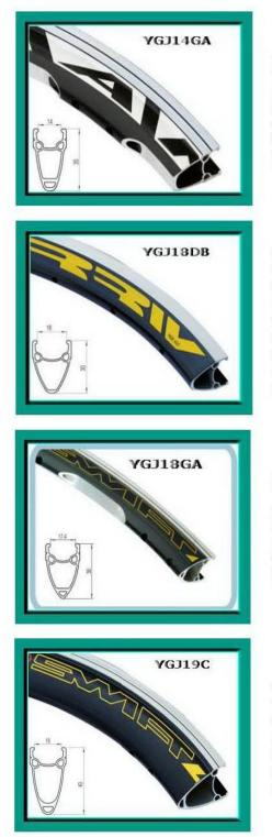
Model: YGJ14GA Tri-layer Height: 35mm Size:700C (ETRTO:622) Holes:24H.28H.32H.36H Finish: Power coating/anodizing Optional: Ground, CNC Side walls
