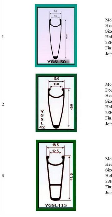
Model: YGSL50 Height: 50mm Size:700C (622) Holes:12H.16H.20H.24H. 28H.32H.36H Finish: Power coating Joint: Sleeved
